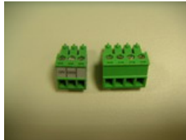
Terminal Blocks for Power & DI/O
